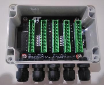
In response to boats suffering instrument failure through water getting into wiring, A+T has introduced the waterproof junction box.
